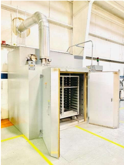
Figure 1: High-capacity annealing oven purchased and used to enhance crystallinity and moisture resistance in Delrin-molded parts, ensuring dimensional stability and durability for outdoor applications.
